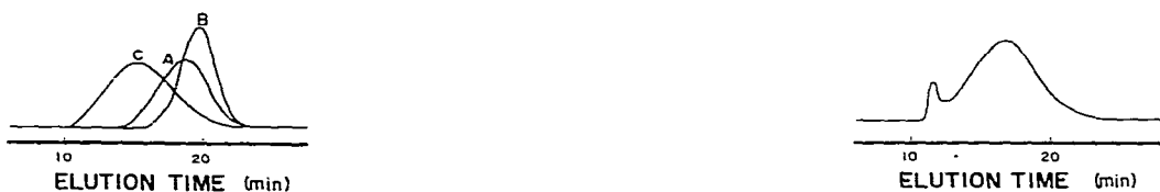
Fig. 14. Chromatogram of three kinds of commercial sodium chondroitin sulphate. Sample: A = sodium chondroitin sulphate A (whale cartilage); B = sodium chondroitin sulphate B (pig skin); C = sodium chondroitin sulphate C (shark cartilage). Column: G 4000 SW. Solvent: 0.1 M NaCl aqueous solution. Pressure: 20 kg/cm 2 . Flow-rate: 1.0 ml/min; charge: 500 \mu l. Detector: RI \times 16. Room temperature.
